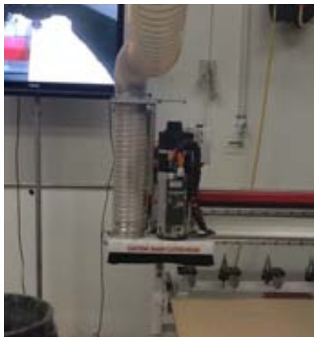
The CNC router in action, cutting out a name plate.
